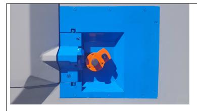
The bending system is provided with a rotating disk that rotates in one direction via servo-motor. On the disk, a side bending pin is placed, which has the ability either to move towards the centre of the disk or to move back towards the periphery of the disk, depending on the diameter of the rod to be elaborated.
