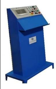
The control panel is installed next to the machine and at its inner part there is an industrial PC. At the front view of the control panel, are adjusted the buttons for manual commands, and the touch screen.
