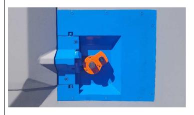
The bending system is provided with a rotating disk that rotates in one direction via servo-motor. On the disk, a side bending pin is placed, which has the ability either to move towards the centre of the disk or to move back towards the periphery of the disk, depending on the diameter of the rod to be elaborated.
