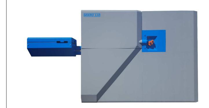
Automatic forming machine from coil, uni-directional, programmable, CNC, designed for the production of common stirrups as well as the re-bar bending.
