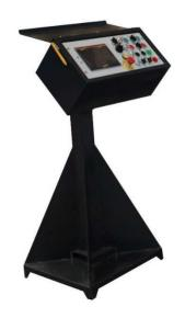
The control panel is placed next to the machine and at its inner part there is an industrial PC.
